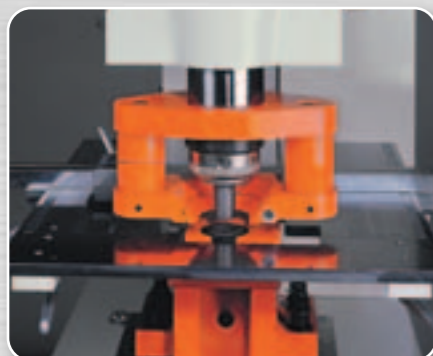
*Urethane spring stripper for minimal deformation.
